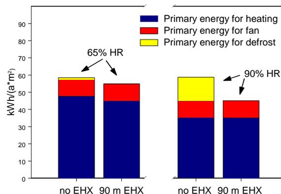
Fig. 7. Simulation results of primary energy demand for two different heat recovery efficiencies with (case 3) and without (case 2) an earth heat exchanger in Stockholm (S).
