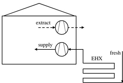
**Fig. 2.** Layout of the ventilation system with earth heat exchanger (Case 1).
