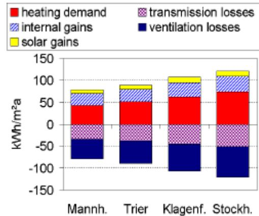
**Fig. 5.** Energy balance of the sample building for the reference case (see Fig. 1) for four different locations.
