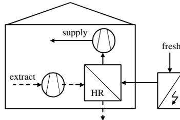
**Fig. 3.** Layout of a balanced ventilation system with heat recovery. A defroster is used to prevent freezing in the heat exchanger (Case 2).
