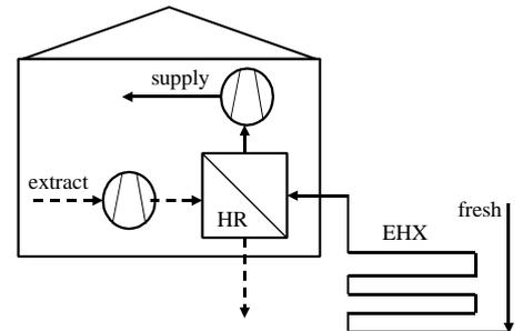
**Fig. 4.** Layout of a system combining both, heat recovery unit and earth heat exchanger (Case 3).
