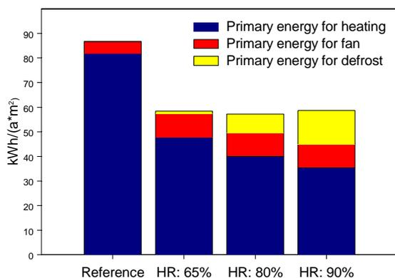
Fig. 6. Simulation results of primary energy demand for the reference case compared to systems with different heat recovery efficiencies (case 2) in Stockholm (S).
