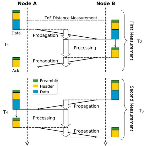
Fig. 2. Symmetrical Double-Sided Two Way Ranging [18]
