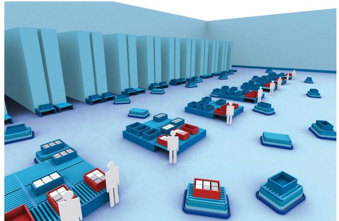
Fig. 1. Swarm of mobile robots in a distribution center © Fraunhofer IML
