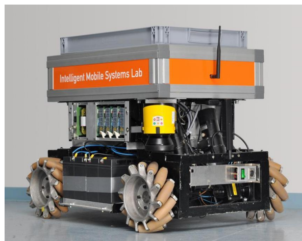
Fig. 1. Omnidirectional transport robot
