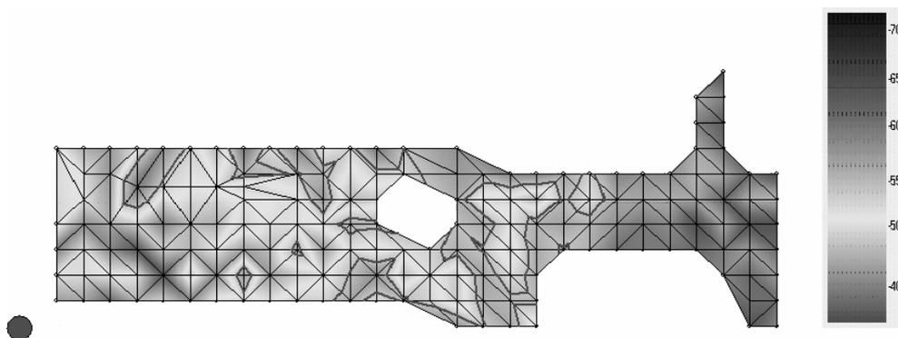
Figure 5: Radio map with lines of constant signal strength (isobars)
